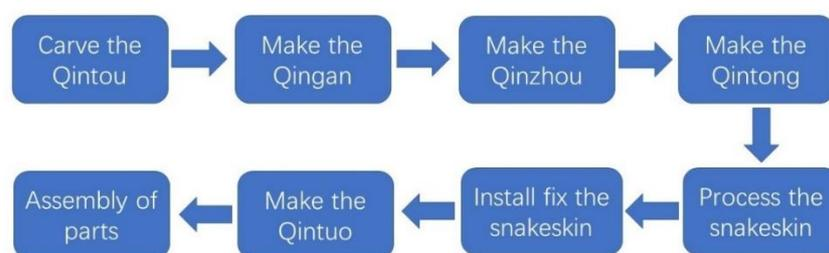
Figure 1. Flowchart of making stringed instruments
